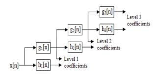
Fig 2: Decomposition of Stationary wavelet Transformation
