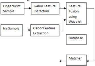
Fig 1 Block diagram of a Multimodal biometric
