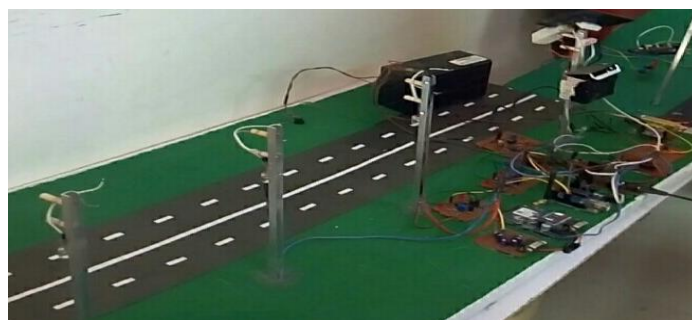
Fig. 2 experimental setup of hybrid and secured solar street light system
