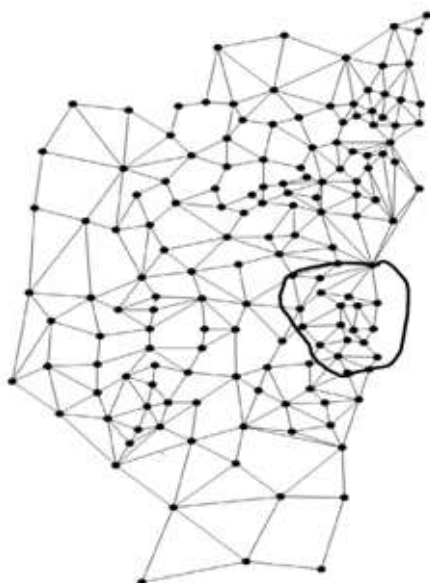
Fig. 2: The graph obtained by the Teynampet zone (highlighted), where each vertices represents the wards and the edges represents their adjacency.
