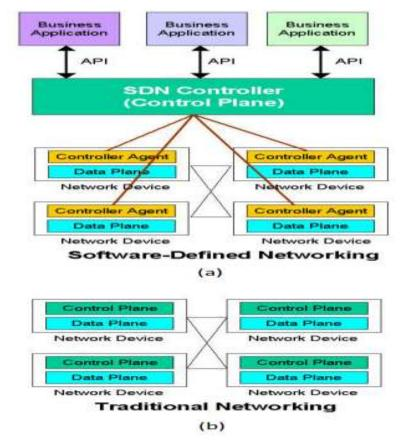
Figure 1: Comparison between the architectures of (a) traditional network; (b) SDN network
