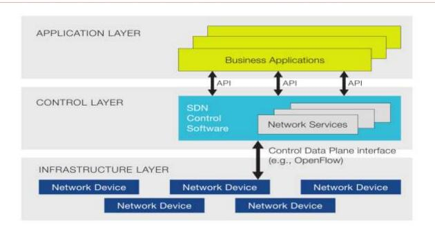
Figure 2: Main layers of SDN architecture
