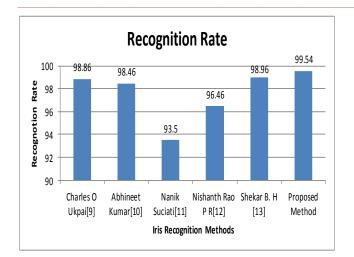
Comparison of Iris Recognition rate with Conventional Algorithms and Proposed algorithm
