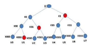
Figure: The NNL tree for broadcast encryption for 8 users. Each K represents an independent cryptographic key. Each user Uj receives all the keys on the path from the root to their leaf node. To encrypt the data, encrypt a copy of the data under the keys at the roots of sub trees containing only authorized users. For example, to encrypt to the set of all users except U0, one would use the keys corresponding to the nodes colored in red.
