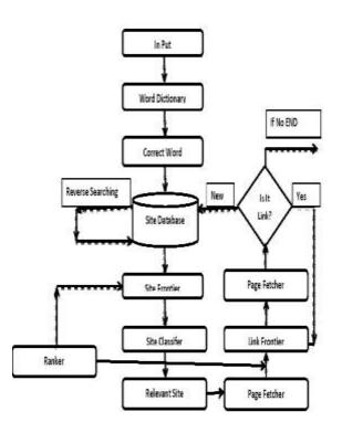
Fig. 2. System Architecture for Hidden(Deep) Web Crawling
