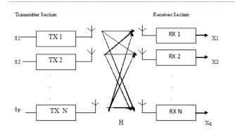
Fig.2.1 A schematic representation of MIMO antenna
