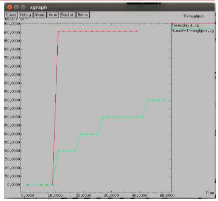
Figure 7.2: Comparison of proposed scheme and M-LEACH with respect to throughput.
