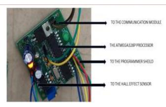
Figure 4. Fabricated PCB
