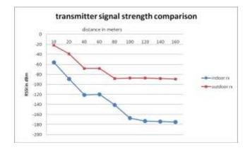
Figure 8. Signal strength -range analysis of transmitter
