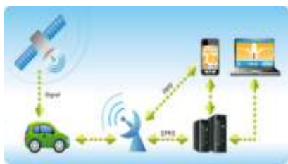
Fig. 2 Vehicle Tracking System using GSM & GPS.
