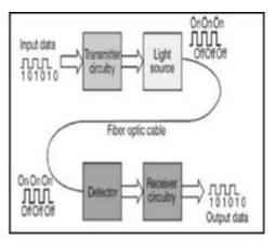
Figure 3: Basic Optical Fibre Communication [8]
