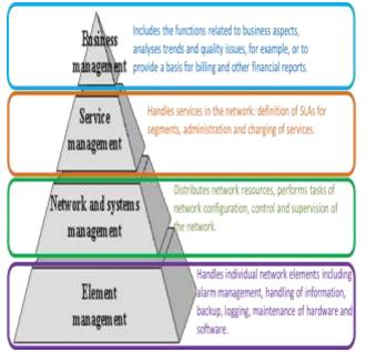
Figure 2 :- Architecture of 1350 optical management system
