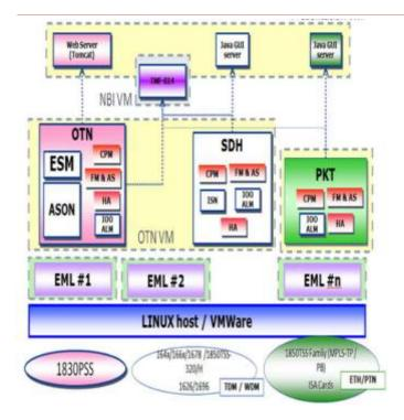
Figure 3: - 1350 OMS Management Layers, Technologies, and Applications
