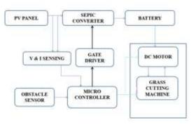
Figure 1.Block diagram of the proposed system.
