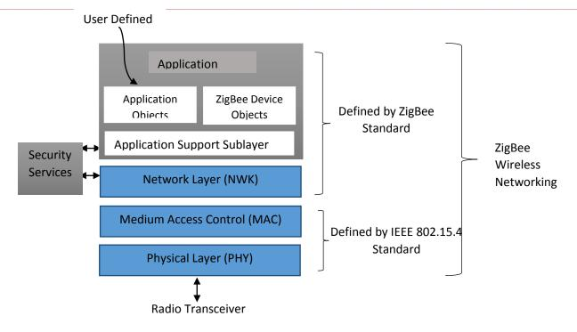
Fig 1: Relation between ZigBee and IEEE 802.15.4
