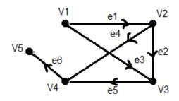
Then we can take an incidence matrix of G is Q(G) of  $n \times m$ . The row and column of Q(G) is 0. If vertex *i* and edges  $e_j$  are not incident other wise it is 1 or -1 for example fig.
