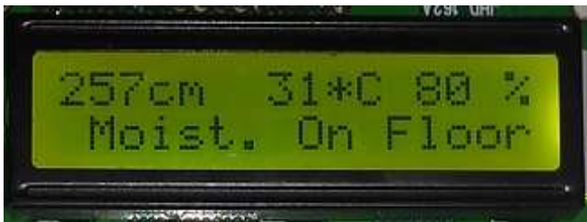
Fig 6: Moisture is detected through the water sensor.
