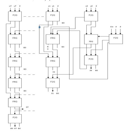
Fig. 7: First Proposed Architecture of Reversible 8-bit Parity Preserving CLA Adder Circuit
