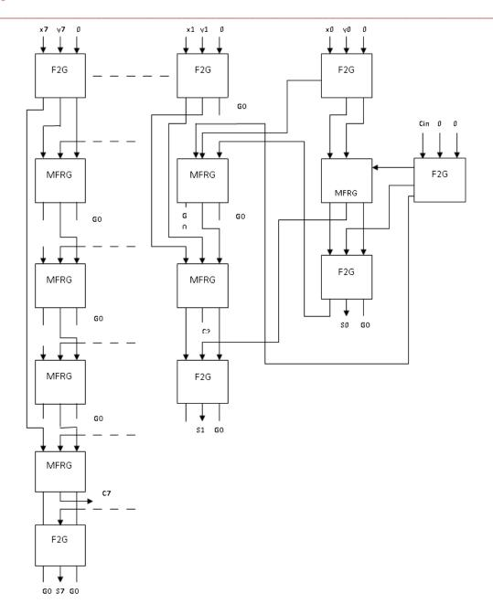
Fig. 8: Second Proposed Architecture of Reversible 8-bit Parity Preserving CLA Adder Circuit
