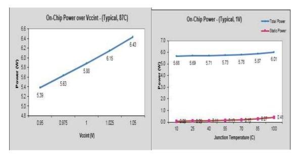
Fig. 13:Power Dissipation Graph for Proposed Reversible Parity Preserving CLA Circuit (Architecture 1st)
