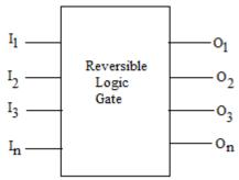
Fig. 1. Symbol of Reversible logic gate with n\*n input and output
