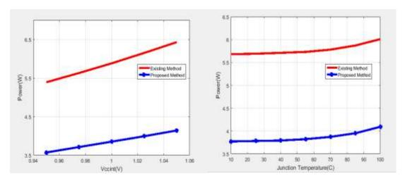
Fig. 15: Comparative Results of Power Dissipation Graph for First Proposed Architecture&Second Proposed Architecture of Reversible Parity Preserving CLA Adder Circuit
