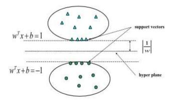
Fig.5 A linear separable Support Vector Machine
