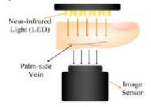
Fig. 1 Finger vein imaging (Light Transmission method)
