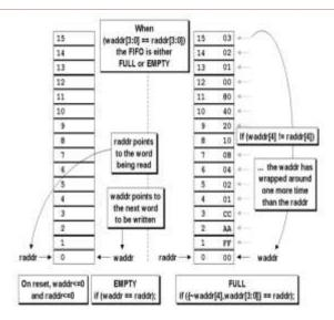
Fig 7. FIFO full and empty conditions
