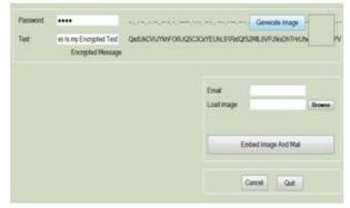
Fig. 5 Text has converted to MORSE code then encrypted using password as key
