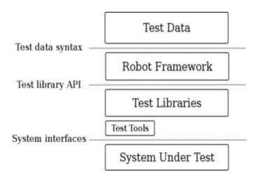
Figure 1. Robot Framework architecture
