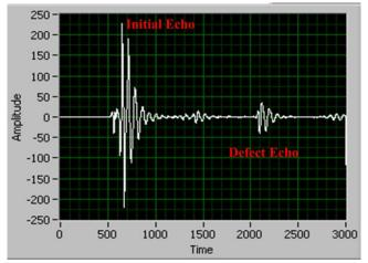
Figure 4: A-Scan signal obtained from the defect location in the welded region (angle beam technique).
