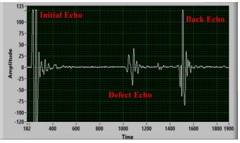
Figure 3: A-Scan signal obtained from the defect location in the welded region (normal beam technique).
