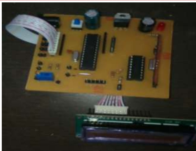
Figure 8: Hardware implementation of heart rate measurement device (Receiving part)
