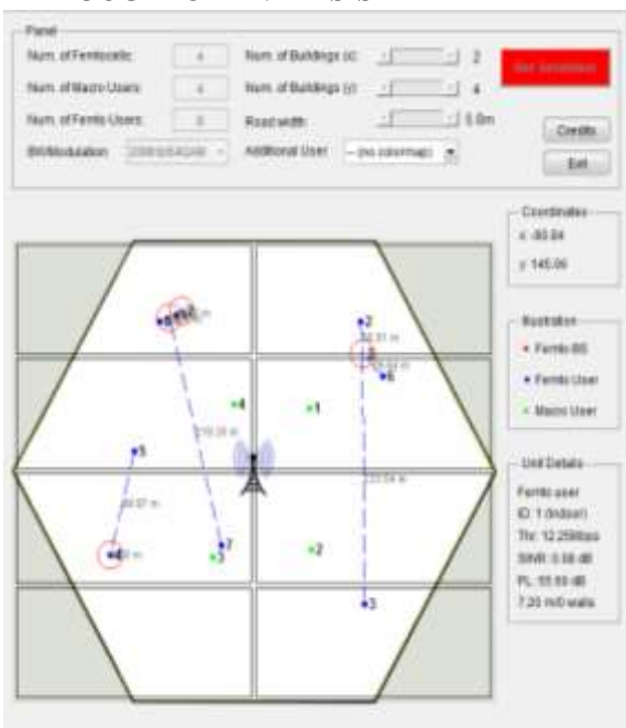
Figure 5.4 Placing of Femto and macro users in a cell and throughput of a femto user
