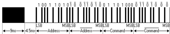
Figure 7. Message frame using the NEC protocol.
