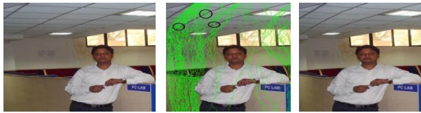
Fig 5: (a) Original Image with resolution 800 x 600, (b) Image after applying seam carving algorithm with improvement (Dark black circle represent intersection of multiple seam over a single point on straight line (c) image after applying seam carving algorithm without showing seam over the image, This image shows the distortion of straight line.
