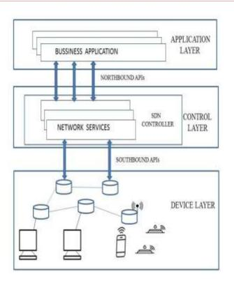
Figure1: Layered SDN Architecture
