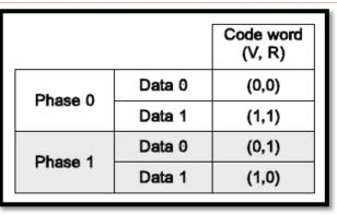
Figure 7. LEDR encoding
