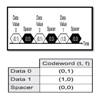
Figure 6. 4 phase dual Rail Encoding
