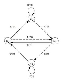
Figure 2: State Diagram of Encoder
