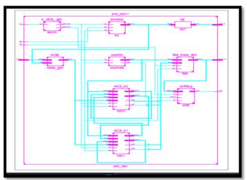
Figure 8 RTL View of Asynchronous Viterbi Decoder
