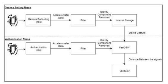
Figure 1. System Architecture
