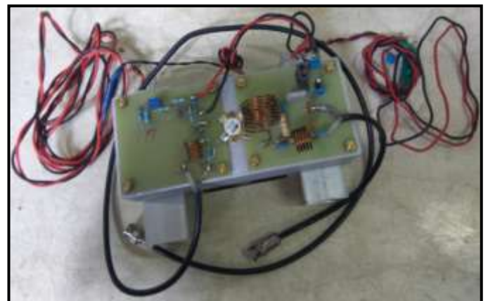
Figure 14: Circuit fabricated with low pass type of the output matching circuit
