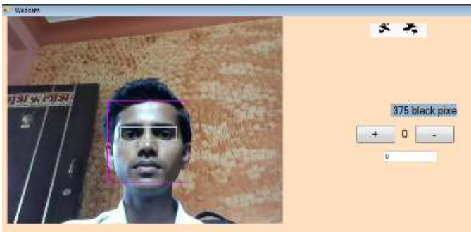
Fig.11(h): Face captured; eyes detected and open; therefore alarm not sounded
