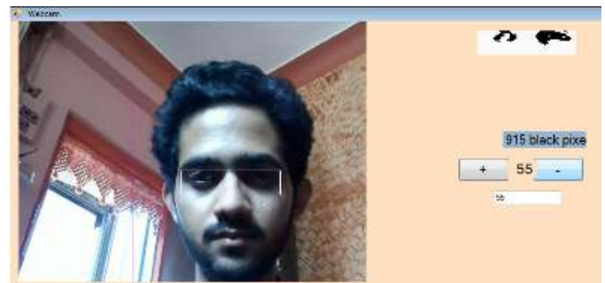
Fig.11(d): eyes detected and open; speed is 55, therefore alarm not sounded because speed is within the threshold
