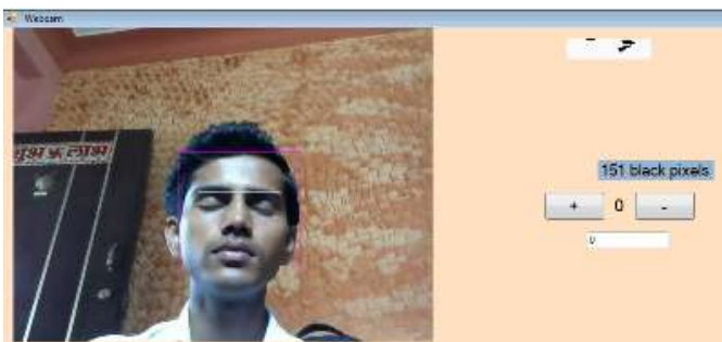
Fig.11(i): eyes detected but they are closed, so alarm is sounded
