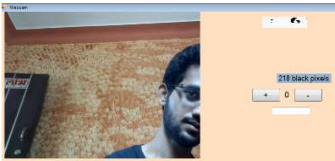
Fig.11(g): face not captured as the person avoids the camera, but then also alarm is sounded.
