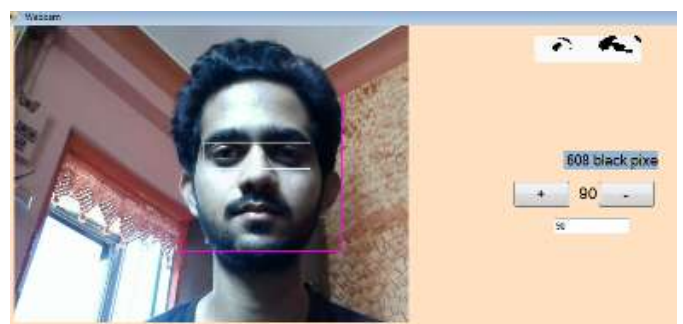
Fig.11(e): eye region captured; speed reaches limit but alarm will sound only after speed>90
