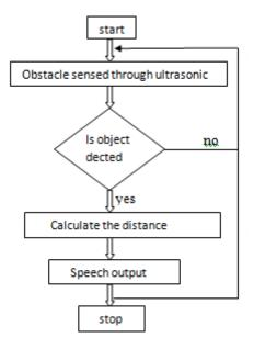
Our project is an innovative idea of intelligent system which has basically Obstacle detection feature and will provide safety and support to visually impaired Persons. The ultrasonic sensors in the system will sense surround-ing and will detect the obstacles and give feedback to raspberry pi speech synthesizer change the path way.
