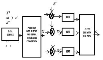
Figure 2: The Block Diagram of Selected Mapping Technique [12]
