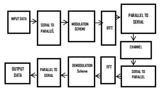
Figure 1: Block diagram of an OFDM system [13]
