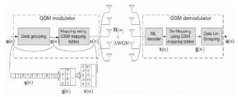
Fig. 1Generalised spatial modulation system model. At each instant four bits are transmitted. Three bits are encoded in the indices of the combination of transmit antennas and one bit is conveyed inthe signaldomain using BPSK modulation.
