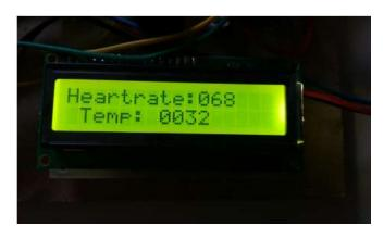
Figure 2. Heart rate & Body Temperature displayed on LCD Display
