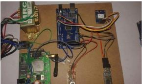
Fig.4 Hardware of Bike Dashboard Unit
