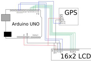
Fig.2 GPS and LCD are connected with ARDUINO
