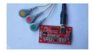
Figure: 4.a ECG SENSOR
