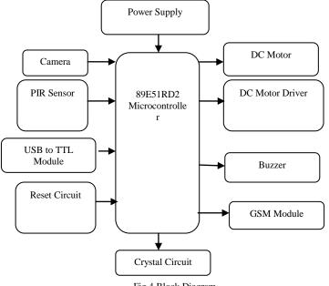
Fig.4 Block Diagram
