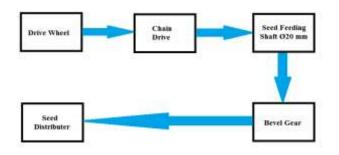
Figure 5.2: Energy Flow Diagram for Seed Sowing.
