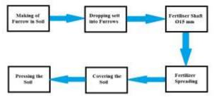
Figure 5.1: Flowchart Showing Sequence of Operations
