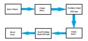
Figure 5.1.1: Energy Flow Diagram for Sugarcane
