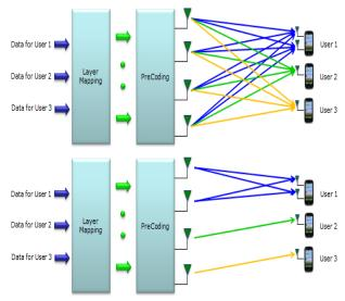
Fig 4. Different Antenna allocation Modes
