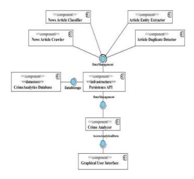
Fig. 1.  $\Box$  High level architecture of the proposed system
