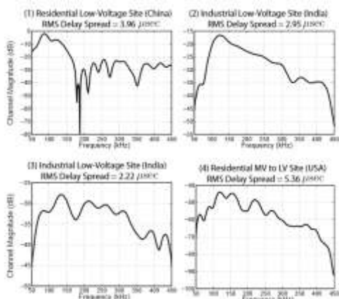
Fig. 1. Examples of different PLC channels in frequency domain and their corresponding RMS delay spreads
