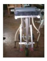
figure 4: machine of seed sowing.
