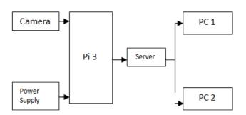
Fig. 1 System Architecture
