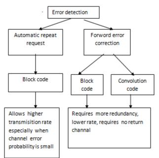
Figure 1.2: Overall classification of error detection & correction schemes [1]
