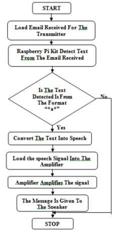
Fig. 6 Flowchart for Receiver
