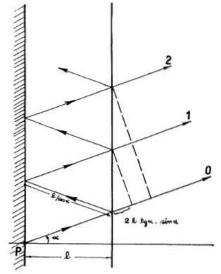
Figure 3. Multiple reflections between PRS and ground plane [6]
