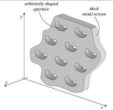
Figure.5- Thick perforated metal screen with arbitrarily shaped aperture [18]
