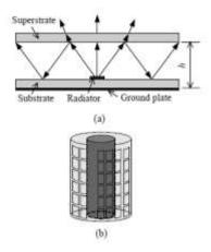
Figure 2(a). Geometry of planar type FPRA (b) Geometry of cylindrical type FPRA [1]
