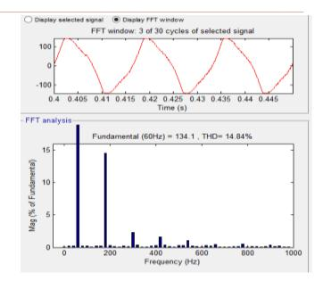
Figure 4. THD when unidirectional ac- dc boost converter connected applying PI controller
