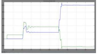
Figure 6. Active power and reactive power when PI control is applied.
