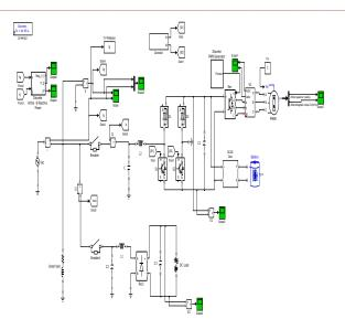
Figure 1.Simulation model for power quality improvement using unidirectional ac -dc boost converter
