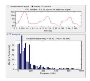
Figure 3. THD without connecting unidirectional ac - dc boost converter
