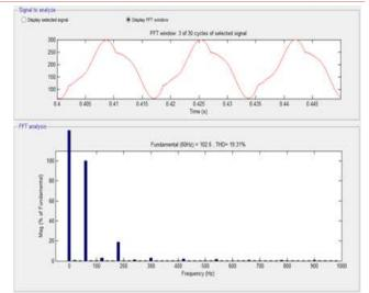
Figure 7. THD when unidirectional ac– dc boost converter connected applying PID controller
